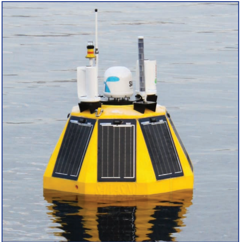
Floating APB5 buoy near Bergen, Norway, with solar panels, wind generators and embedded Web server.
