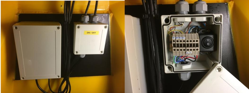
Fig. 4. Power switch box inside the buoy.
