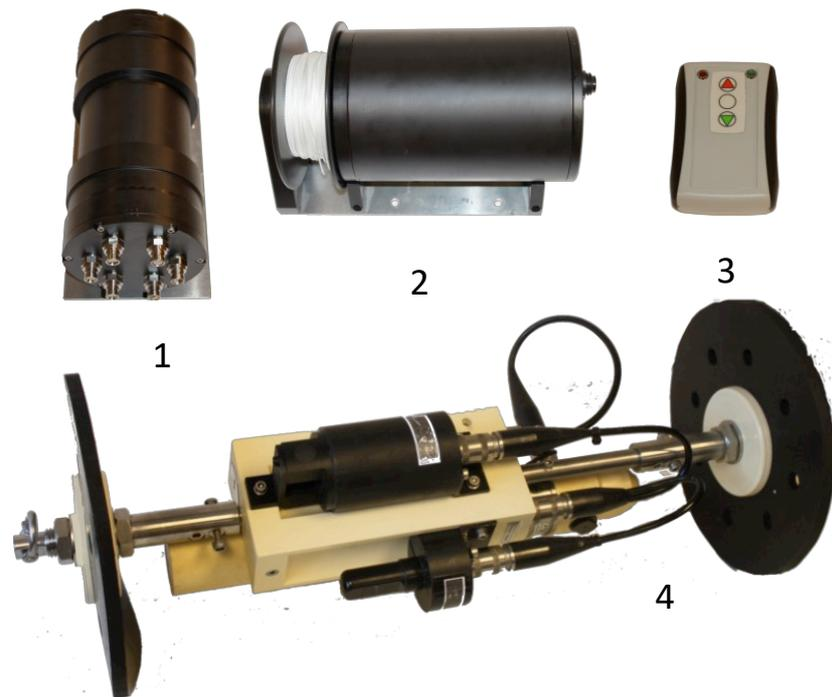
Fig 3. Components of the APB5: 1 = Main electronics (CU801B) and batteries (3 identical cylinders), 2 = Winch, 3 = Remote control, 4 = CTD with optional sensors and protection kit.
