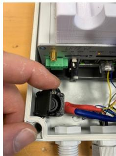
In version 5. Antennas is moved inside the router box, if network has good coverage at the area where the APB5 is placed, is recommended to use the internal antennas. External antenna is mounted on the all APB5, but user only physical connect this if network is poor. Use an 8 mm tool to disconnect the internal antenna and replace it with the cable. Use the ANT (to the left)
