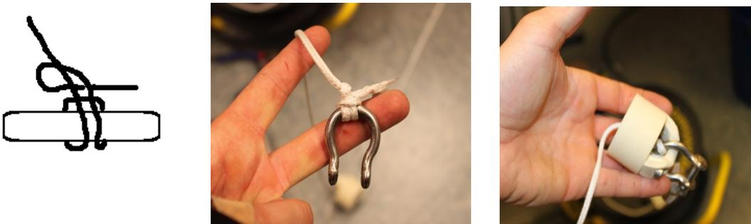
Fig 6. A clove hitch is used to fasten the CTD to the winch rope.
